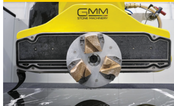
POLISH TOOL Ø 320 mm 3 SEGMENT 36x2 FRANKFURT TEXTURE PLATE
