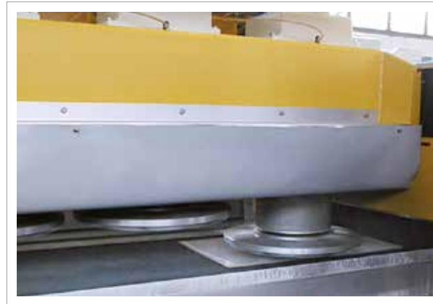
Machine basement with interchangeable stainless steel plates Basamento con piano riportato in acciaio inox
