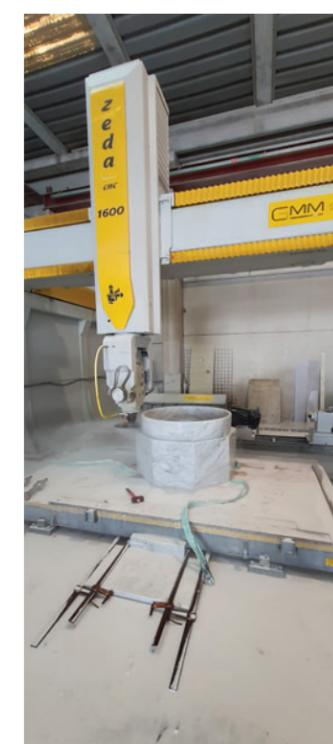
**Cn2** mainly used for slabs cut to size equipped with on-board camera and **Vacuum manipulator, automatic tool change for recessing and holes drilling**.
