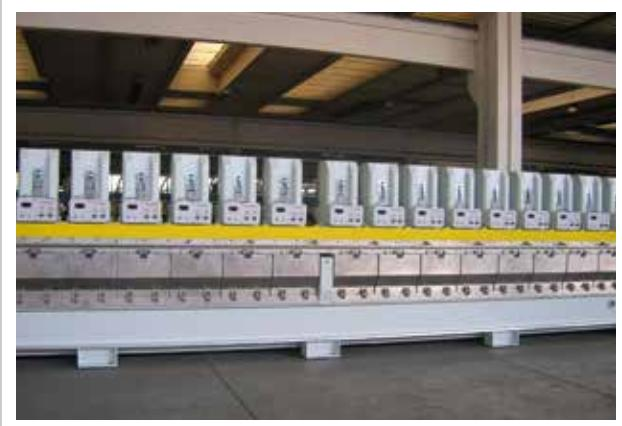
Horizontal diamond calibrating roller for finishing
