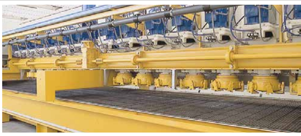
Back view of the central beam carrying the spindles Vista posteriore trave centrale porta mandrini
