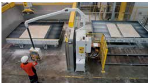
Rapid load/unload system for slab using moving table tops.
