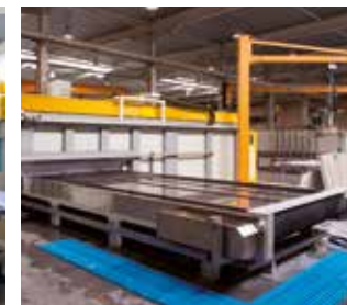
Cutting centre where the stone is transported into the cutting area, and after cutting cycle completes, out of the cutting area by a large dimension heavy duty belt instead of having a standard cutting table.
